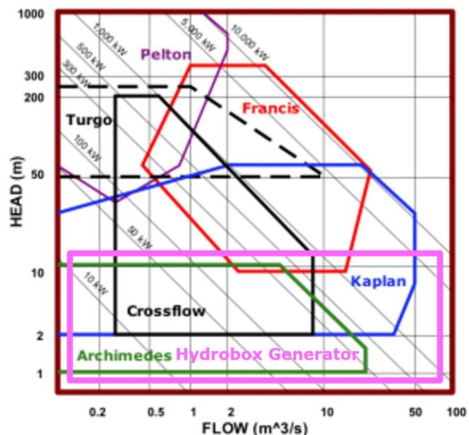
Waterwheels are ideal for the low pressure operations and the diameter can be specified to suit the head height available. Traditional waterwheels have narrow buckets and can only handle low volume flowrates. However, the Hydrobox waterwheel has large segment buckets and the length can be specified to suit the flowrate required.
