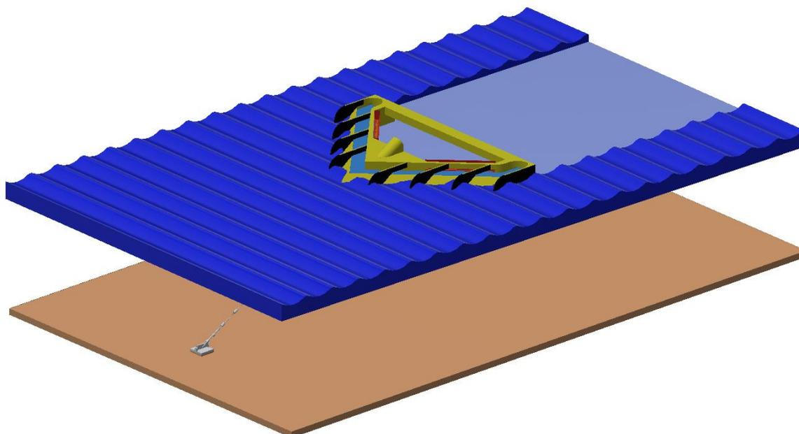
The floating structure weathervanes on its mooring system to always face into the prevailing waves. During operation, the waves travel down both sides of the structure and wash up sloping ramps into an impound reservoir. The stored elevated water is then supplied to a Hydrobox waterwheel to produce electrical power that can then be exported to shore.
