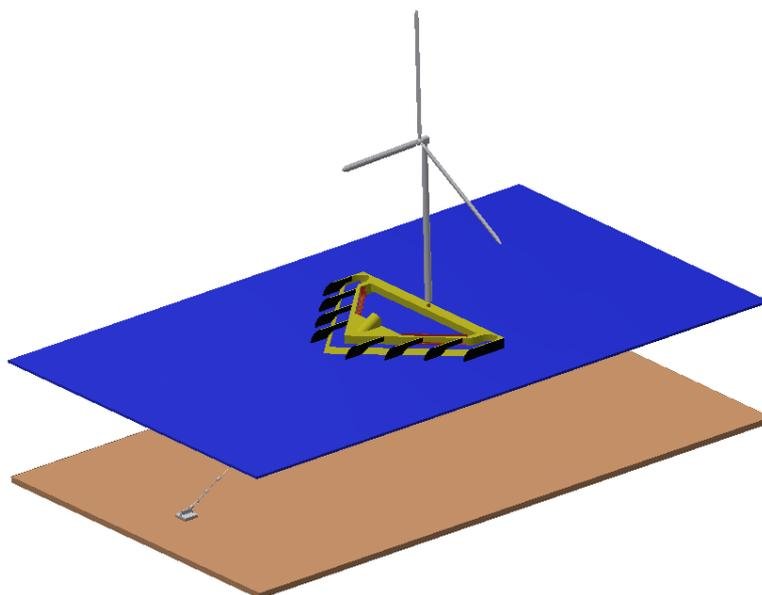
Due to its size, the floating structure will be very stable during operation, this is a requirement for wind turbine performance.
