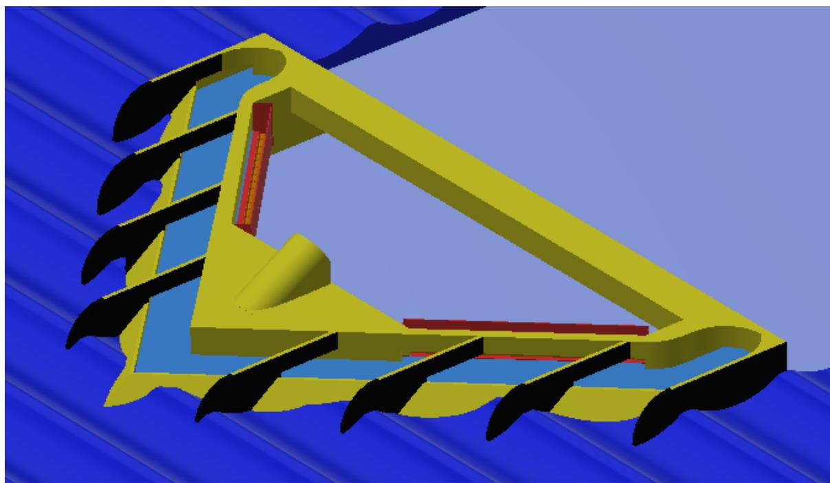
The combination of sloping ramps and elevating guides will maximise the water transferred from the oncoming waves into the impound reservoir.
