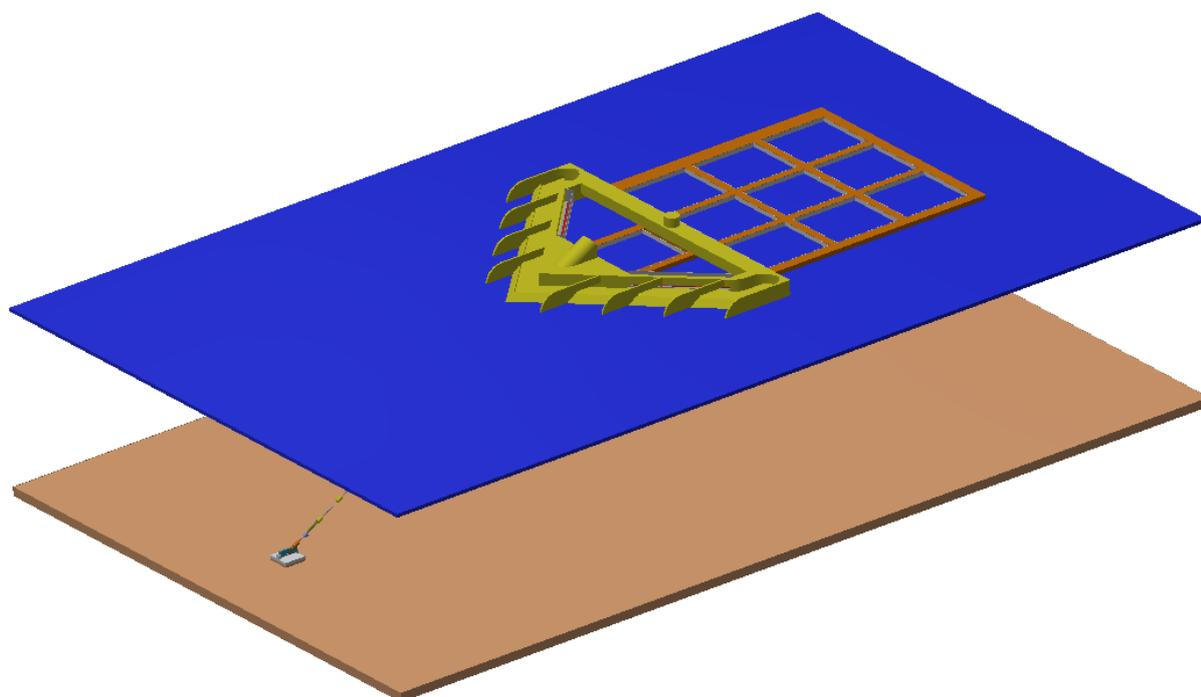
It should be noted that locating the aquaculture system in the calm area astern of the main structure will mean that existing “plastic” cage systems and equipment can be used.
