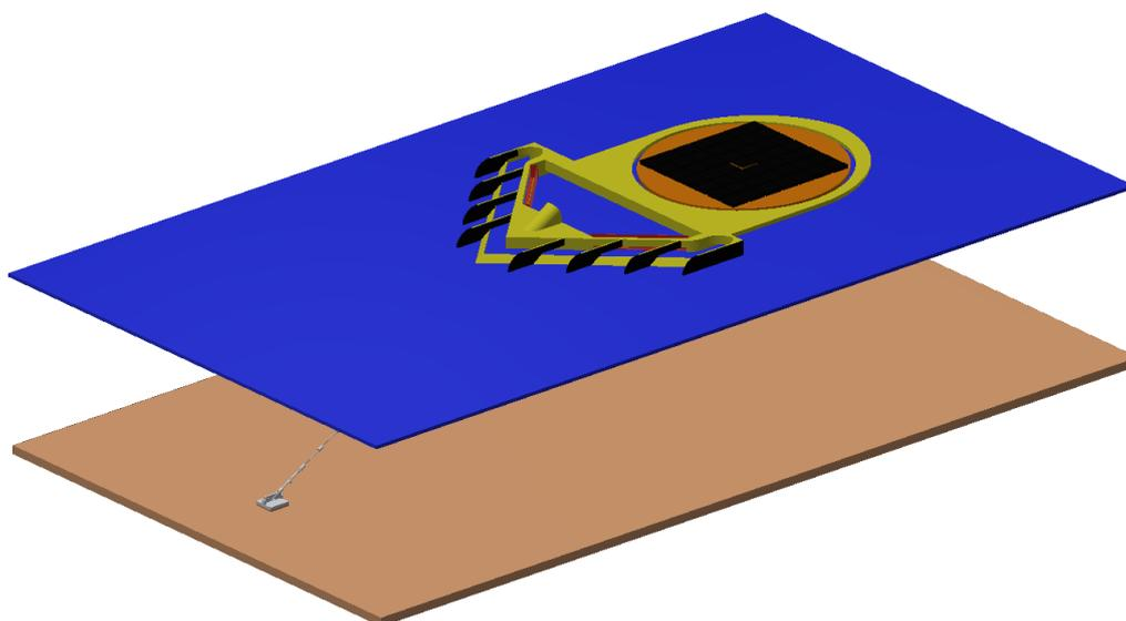
It should be noted that locating the floating solar system in the calm area astern of the main structure will mean that existing “plastic” PV Float systems and equipment can be used. This will remove the requirement for the development of large steel protection structures. The cost effective floating solar systems currently used in inshore lochs, lakes, dams and reservoirs can be use offshore.
