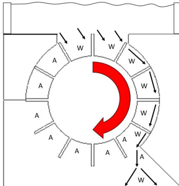
The power generated by the rotor would be dependent on the torque and speed of rotation. An AC Generator would be provided on the rotor end shaft to convert the rotation into electricity.
