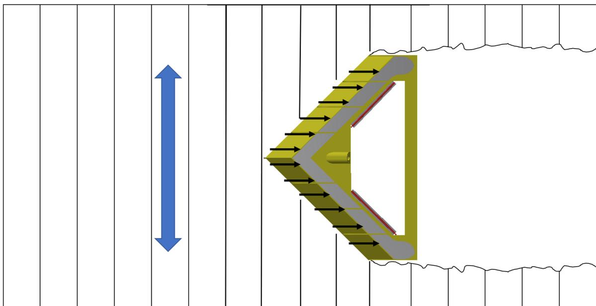
The wave will impact the sloping ramps on the sides of the structure. Due to the energy and momentum in the wave, the water will naturally move up the sloping ramp and into the impound reservoir.
