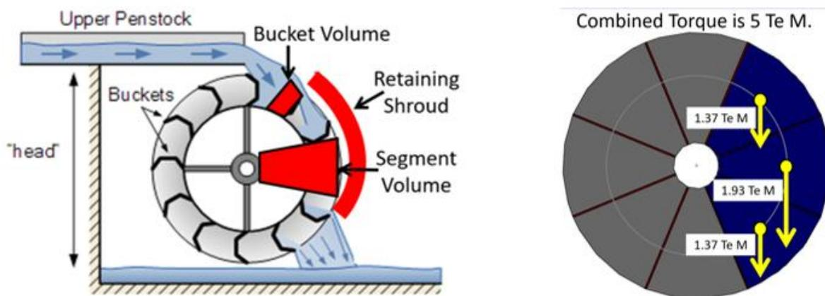
During operation of the Stingray converter, the water in the impound reservoir would be supplied to the inlet at the top of the Hydrobox waterwheel.
