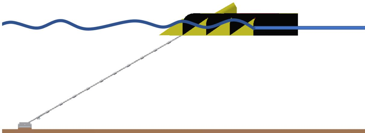
For illustration purposes the Hybrid single line riser mooring system has been used. In this design, the dynamic umbilical is housed within a steel riser pipe for protection. A number of tension chains and buoyancy buoys are configured around the riser pipe. The single mooring assembly is connected to a flexjoint anchor foundation structure on the seabed.
